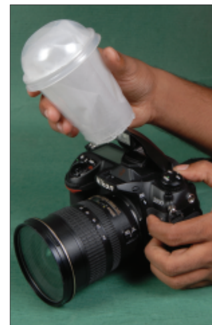
Mount the diffuser properly on the Digi SLR
